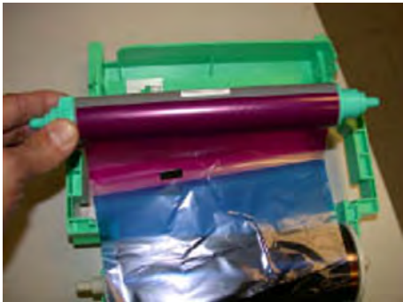
Lift up roll at front.
