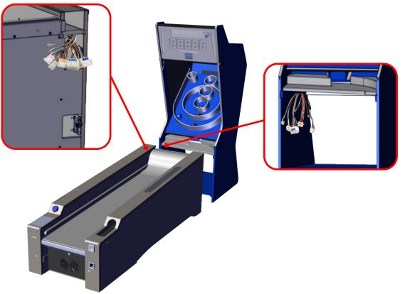
Position the front and back cabinets leaving a space to connect the wire harnesses. Each of the harnesses are color coded. Attach the phone cords together using the provided coupler.
