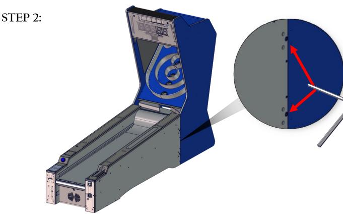
Using the provided latch tool and on both sides of the cabinet insert the tool into the latch openings and turn clockwise until the cabinet pulls together and the locks.
