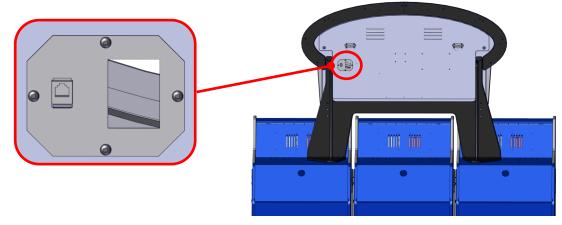
Open the upper Display as described in step 7 and connect the Mega Bonus Linking Phone Cord to any connector not used. It makes no difference which Phone connector on the RGB LED board you use.
