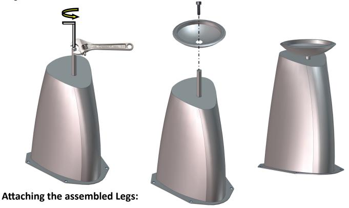
Using four 7/16 bolts and washers attach each leg onto the bottom of the cabinet. Tighten all bolts.
