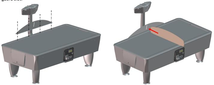
Slide the other side guard into the other end of the playfield divider and attach using AA6032 8x1/2 Hex w/tek screws
